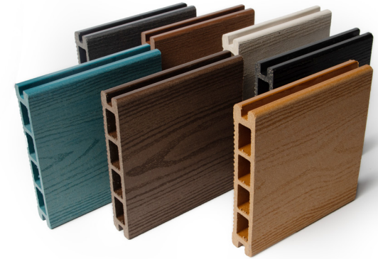
Composite Decking ▲ 5.5" Wide | 1" Thick | 10' up to 20' Long Weight per ft. 1.3 lbs.
